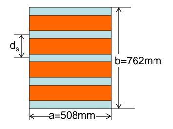
Stiffener geometry and spacing unknown. Determine minimum EI for the stiffeners
