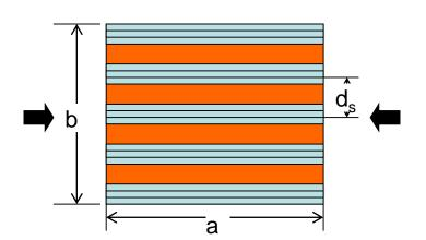
it is assumed the stiffener has an open cross-section and, therefore, GJ≈0
