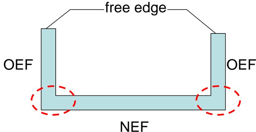
if an edge is not supported or stabilized by another member of the cross-section (or via other means) it is free
