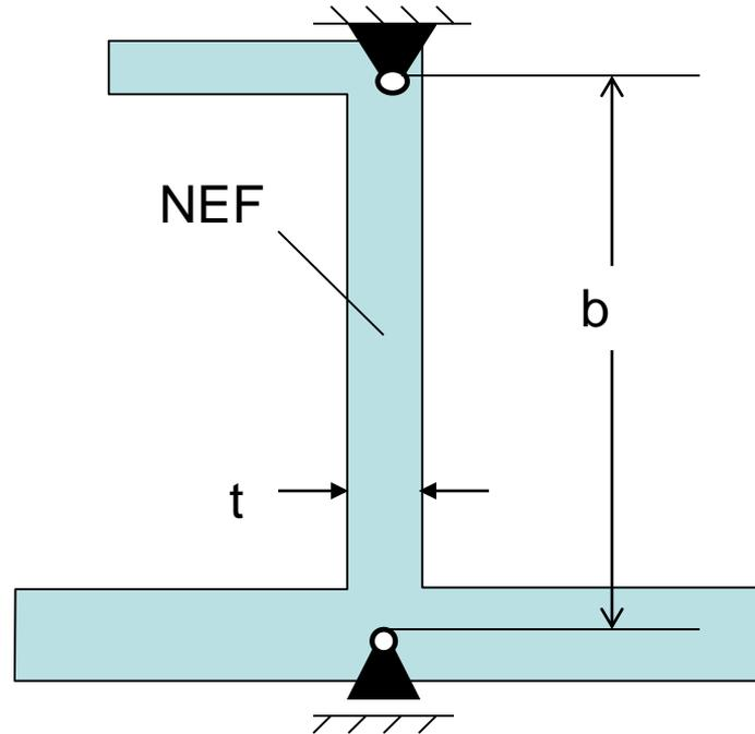
This is the case of a long plate under compression, simply-supported all around which was solved before as part of the biaxially loaded plate
