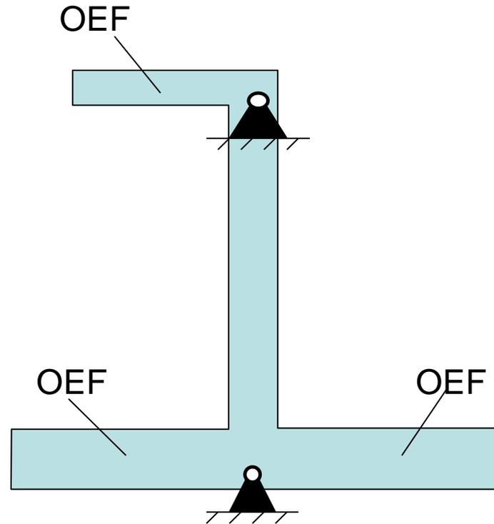
For OEF, the buckling problem has been solved before as the case of a very long plate under compression with three sides simply supported and one side free
