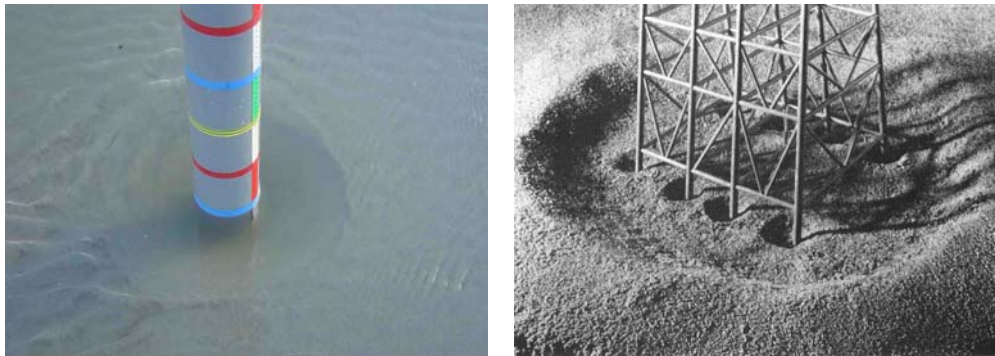
Figure 4 (left) Local scour: steep-sided scour pits around single piles (right) Local and global scour around a jacket structure [2]
