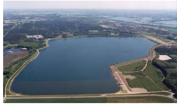
Reservoirbank filtration along a former gravel pit near the Meuse (WML 2004)
