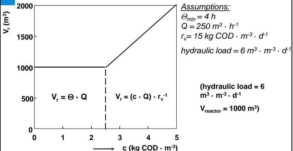
Anaerobic treatment of municipal wastewaters using UASB reactors systems
