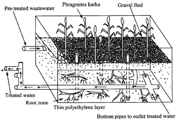
Example of a sub surface constructed wetland, planted with *Phragmites karka*
