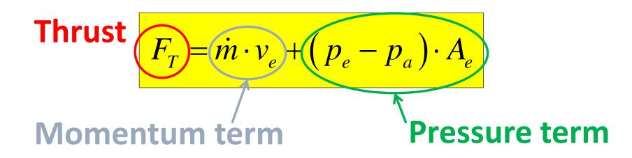
$\dot{m}$  = propellant mass flow rate [kg/s]
