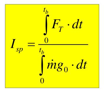
**Definition** of *I*<sub>sp</sub>: <u>total impulse</u> divided by <u>propellant weight</u> Higher  $I_{sp} \rightarrow Less \ propellant$  to deliver same total impulse
