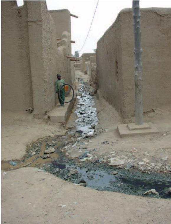
Figure 8 - Accumulation and stagnation of wastewater on the street
