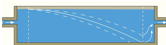
Figure 12 - Influence of turbulence on settling in a horizontal flow settling tank
