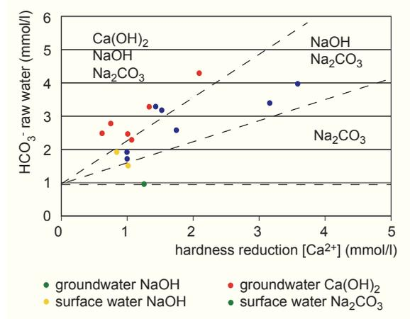
Figure 8 - Application of base as a softening chemical in Dutch practice
