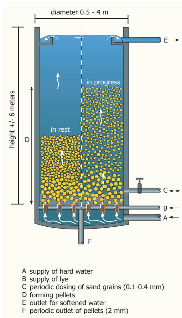
Figure 2 - Schematic representation of a pellet reactor
