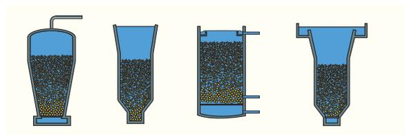
Figure 9 - Different types of reactors
