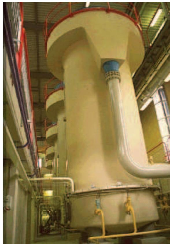
Figure 1 - Pellet reactor used for softening of drinking water
