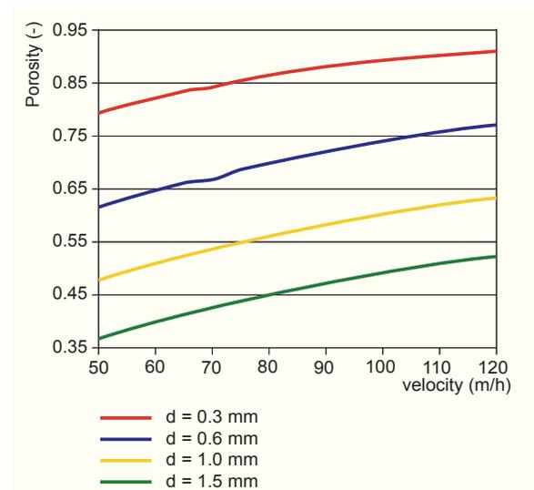
Figure 4 - Porosity as a function of pellet diameter and upward velocity
