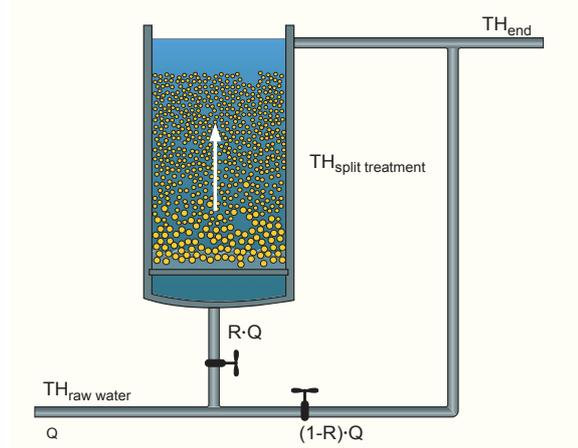
Figure 7 - Principle of split treatment
