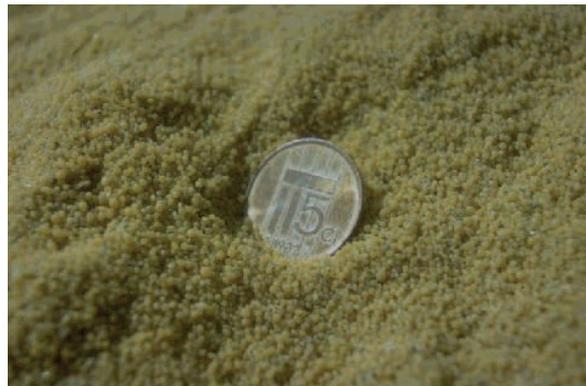
Figure 3 - Limestone pellets
