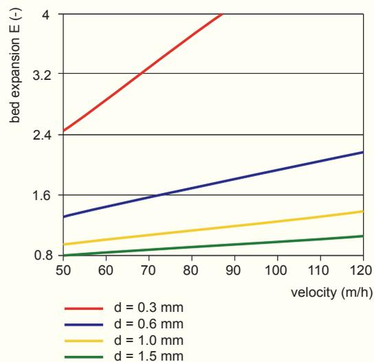
Figure 5 - Bed expansion as a function of pellet diameter and upward velocity
