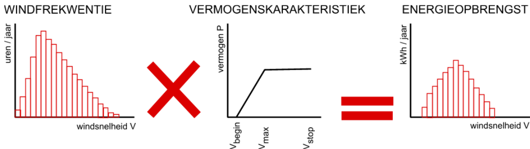
Fig. 232 The way of calculating energy profit of a wind turbine
