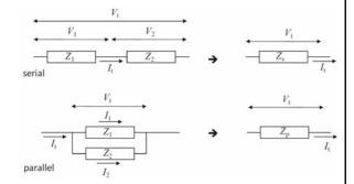
$$Z_{p} = \frac{V_{t}}{I_{t}} = \frac{V_{t}}{I_{1} + I_{2}} = \frac{V_{t}}{\frac{V_{t}}{Z_{1}} + \frac{V_{t}}{Z_{2}}} = \frac{1}{\frac{1}{Z_{1}} + \frac{1}{Z_{2}}}$$
