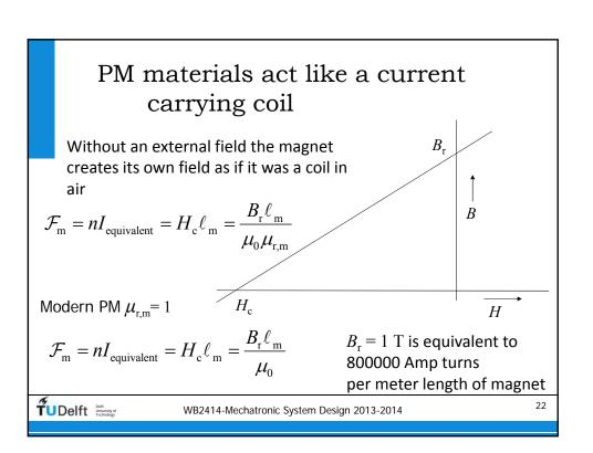
Use a permanent magnet to create a magnetic field in an airgap.
