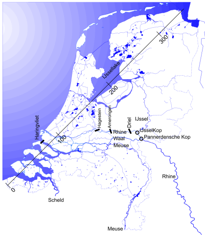
Fig. 441 Weirs directing water northwards and southwards a
