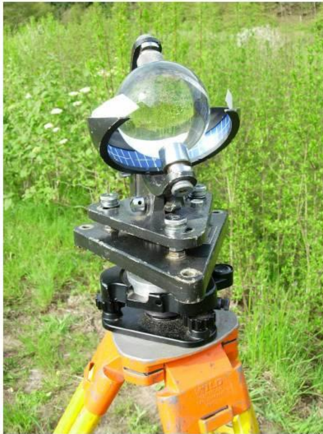
Cambel-Stokes Sunshine duration recorder
