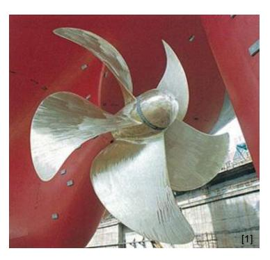
Propulsion Systems – Controllable Pitch Propeller
