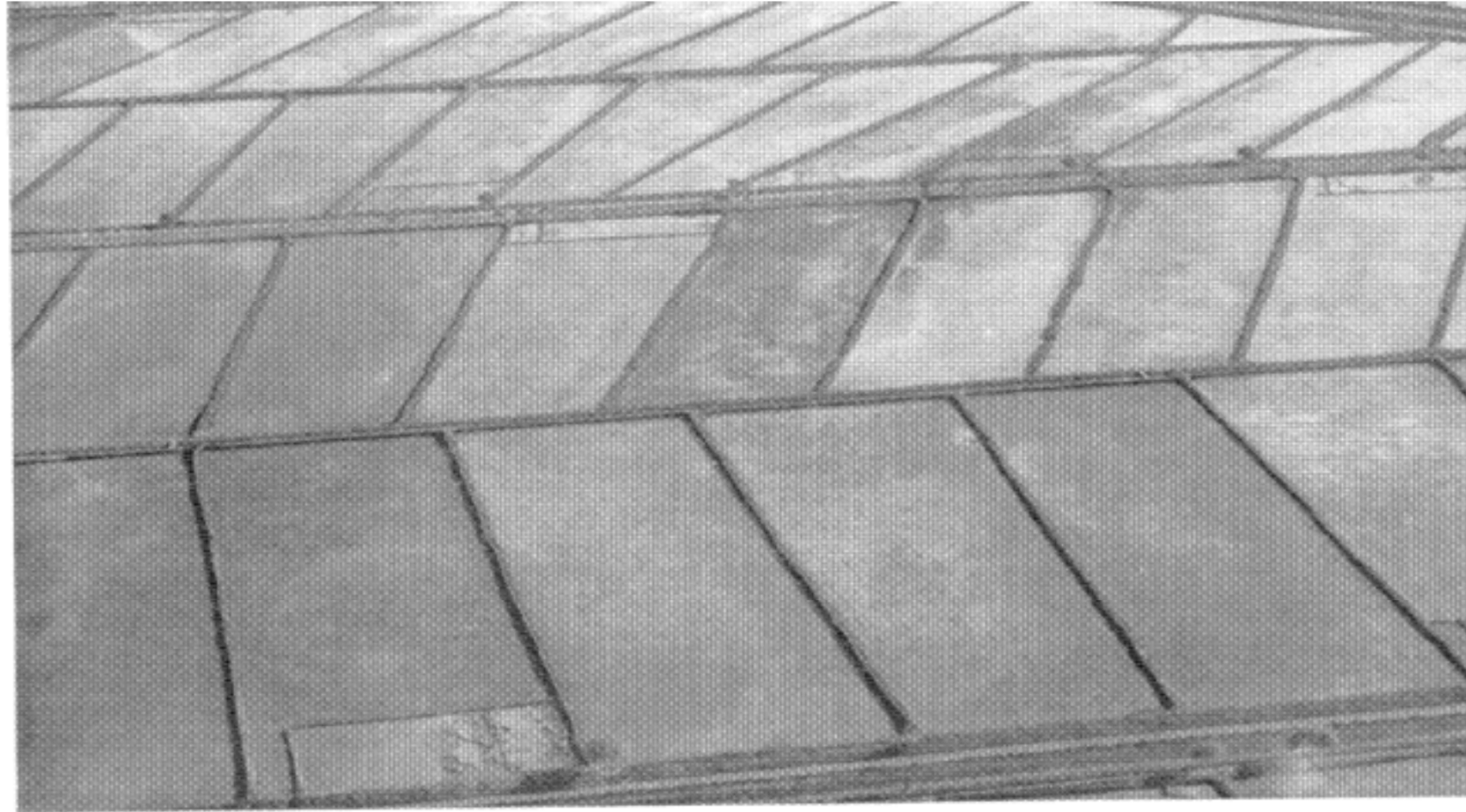
Plate 1. Irrigated paddy fields at Mwea from the air. Note the water control system, with the feeder channels running down the and the drains along the outside next to the roads. Nurseries are visible in the foreground.
