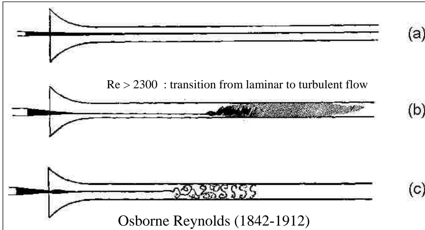
Development of turbulent flow in pipes observed and sketched by Reynolds
