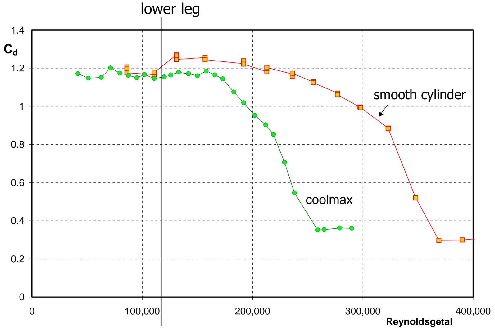
Measured drag characteristics of different fabrics on a cylinder
