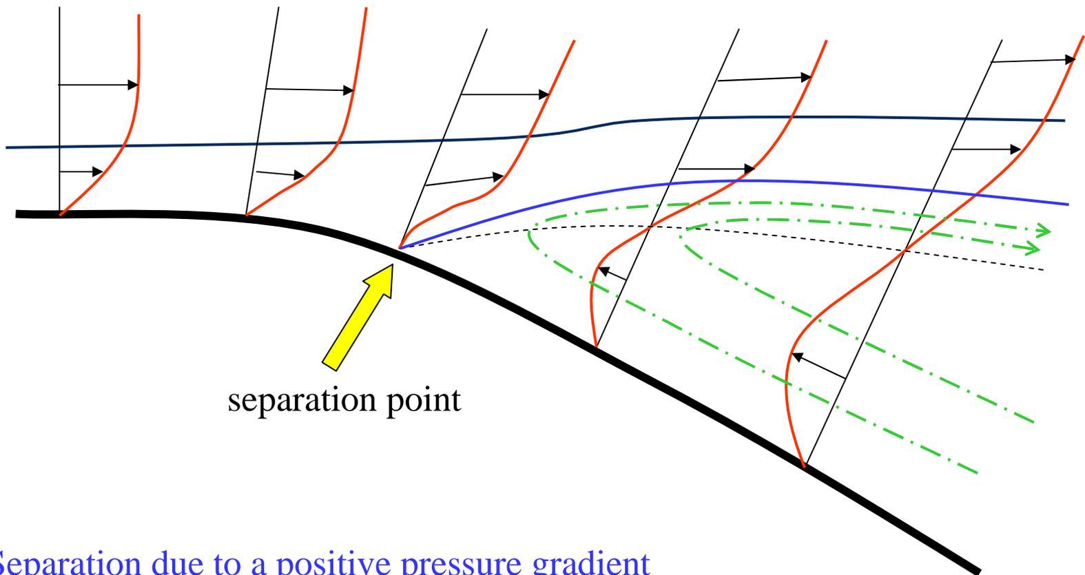
Separation due to a positive pressure gradient
