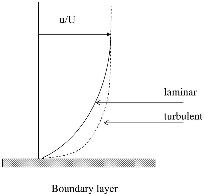
Turbulent boundary layer has more flow **kinetic energy** near the surface. Thus flow separation may be postponed.
