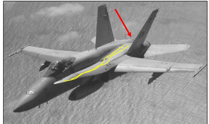
Example : Interaction of separated vortex flow with vertical stabilizer (F18)
