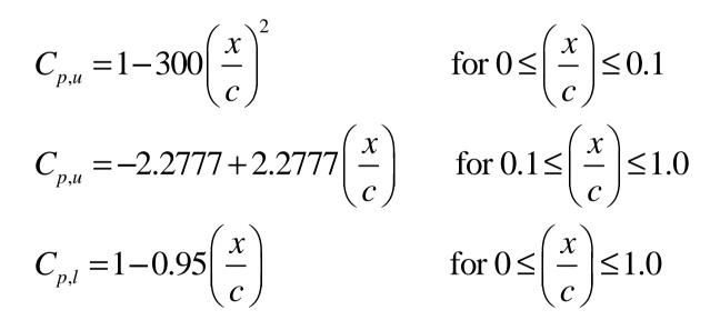
Calculate the normal force coefficient.
