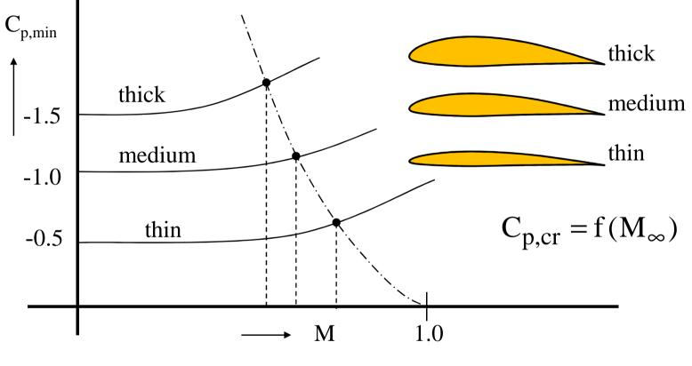
Thicker airfoil reaches critical pressure coefficient at a lower value of  $M_{\infty}$
