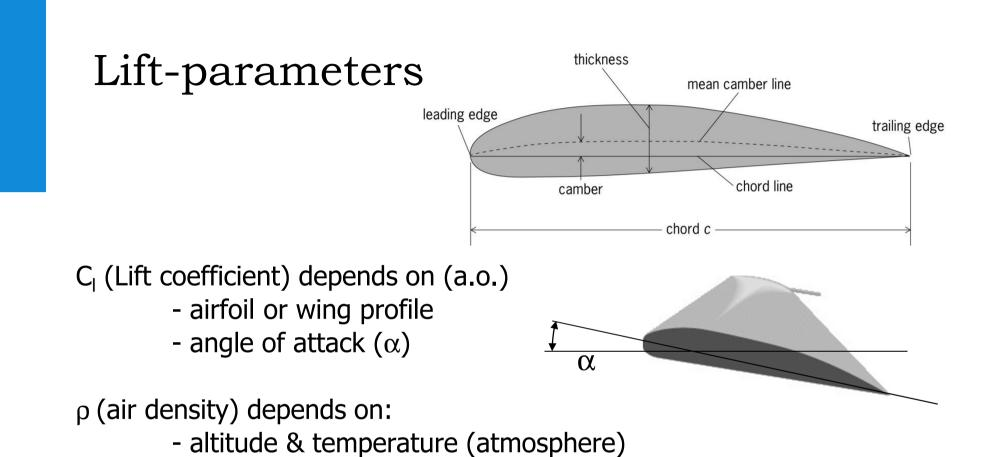
V (air speed) and S (wing area) are design parameters
