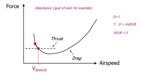
At airspeeds above the minimum drag condition, the aircraft is stable. If the aircraft decelerates (or accelerates) due to a disturbance, then the drag will decrease (or increase). The decreased drag will make the aircraft accelerate (or decelerate). Hence it will return to the original airspeed and is stable.
