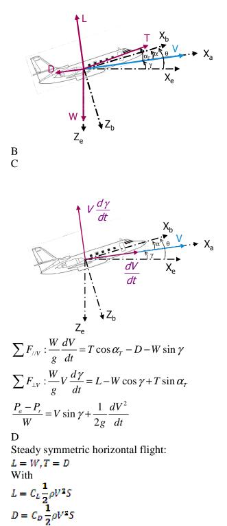
Thrust must be at maximum to achieve  $V_{max}$ . Combining the equations yields:
