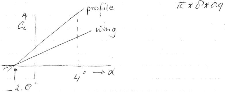
The lift coefficient of the wing follows from :
