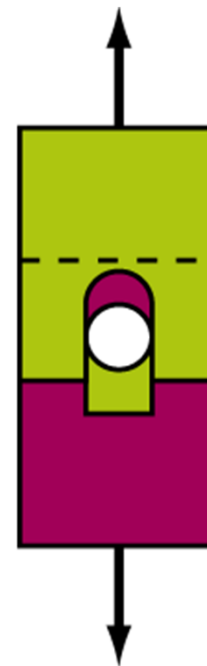
Shear Tear Out
