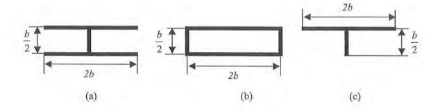
b) Show that the principal moment of inertia of cross-section (c) equals  $I = \frac{17}{480}b^3t$ .
