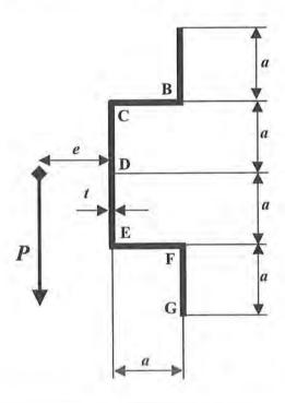
d. Show that the principal moment of inertia for bending due to the shear force P is equal to:  $I = 7\frac{1}{3}a^3t$
