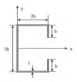
b) Show that the principal moment of inertia for bending  $I = \frac{161}{12}b^3t$ .
