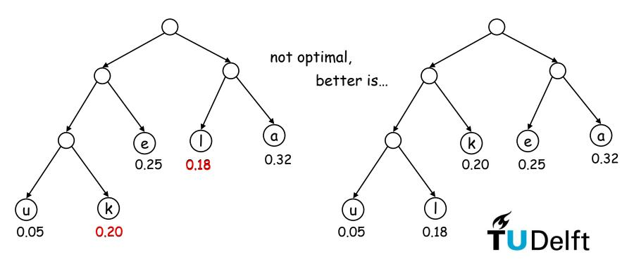
Observation. Lowest frequency items should be at the lowest level in tree of optimal prefix code.
