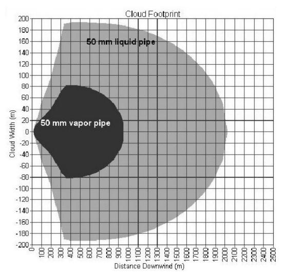
Cloud footprint to an atmospheric concentration of 20 ppm resulting from the rupture of a 50 mm diameter chlorine pipe containing either chlorine liquid or chlorine vapor
