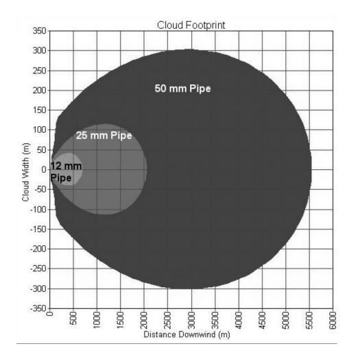
Cloud footprint to atmospheric concentration of 1ppm resulting from the rupture of three sizes of phosgene pipe
