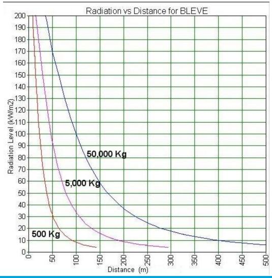
Radiation intensity from a BLEVE (boiling liquid expanding vapor explosion) as a function of distance for propylene storage tanks in three different sizes
