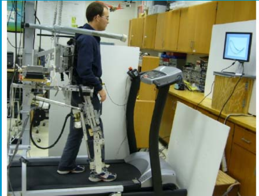
Fig. 2. Gait training exoskeleton on the treadmill, a facility at University of Delaware. The subject walks on a treadmill and the active orthotic device is connected to the right leg. The computer display in front of the subject is for visual feedback of his gait trajectory during training.
