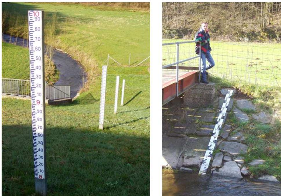
Fig. 6.1: Left: Vertical staff gauge, right: inclined staff gauge
