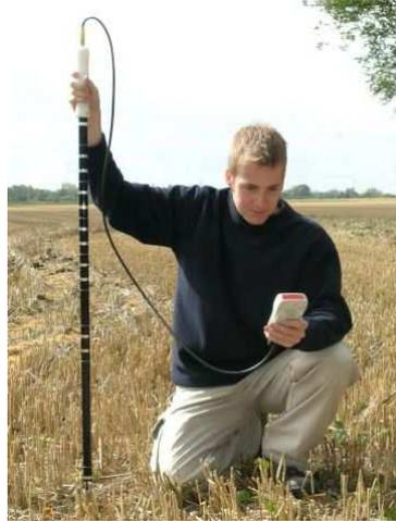
Fig. 5.3: Frequency Domain Reflectometry (*PR2 Profile Probe - Delta-T Devices*)
