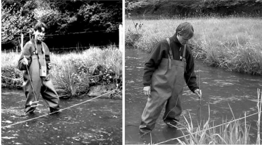
*Fig. 8.12: Current meter by wading*
