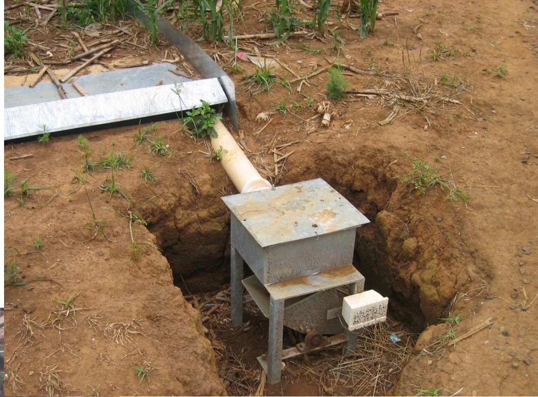
Surface runoff measurement with a tipping bucket, South Africa
