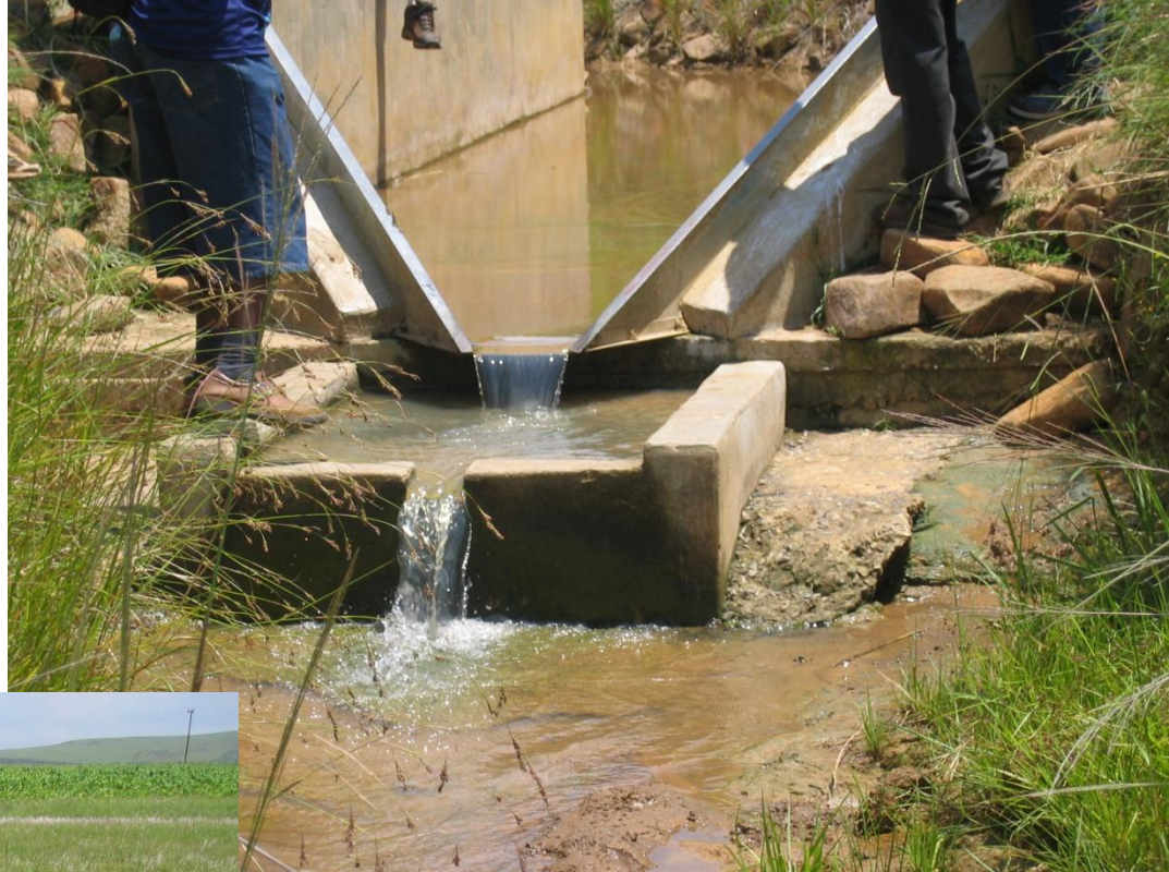
Discharge measurement with a flume, South Africa
