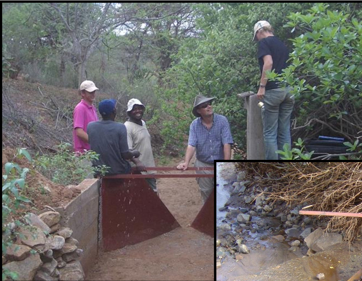
Discharge measurement with flume in an ephemeral stream, Tanzania
