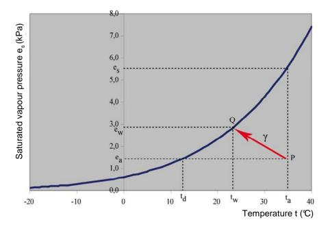
In the figure above you see (an example of) the relation between vapour pressure and temperature. The curved line indicates the saturation vapour pressure as a function of temperature. The relation of the curved line is:
