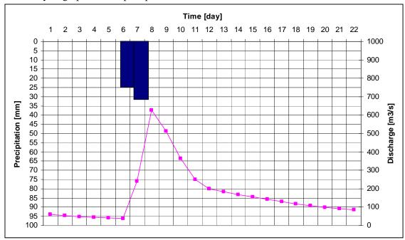
• Discharge has a baseflow and direct flow component. Direct flow ends at day 12. Apply the 'straight line' method to divide the base flow from the direct flow.
