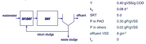
The wastewater is treated with the above activated sludge plant optimized for Bio-P removal. Other required kinetic parameters and process values are tabulated above.
