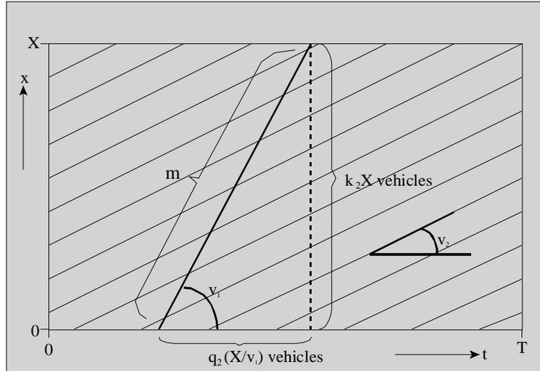
Figure 3.21: Schematised vehicle trajectories to determine number of overtakings
