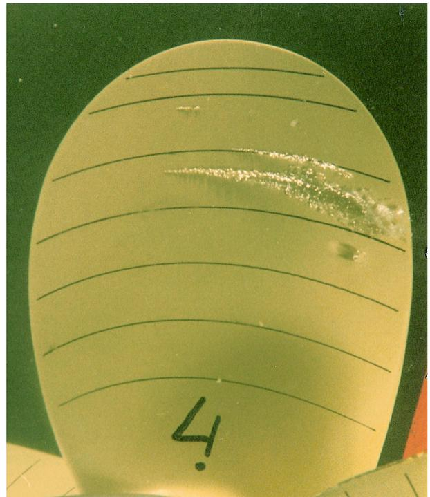
Figure 7.10: Bubble cavitation due to a turbulent spot
