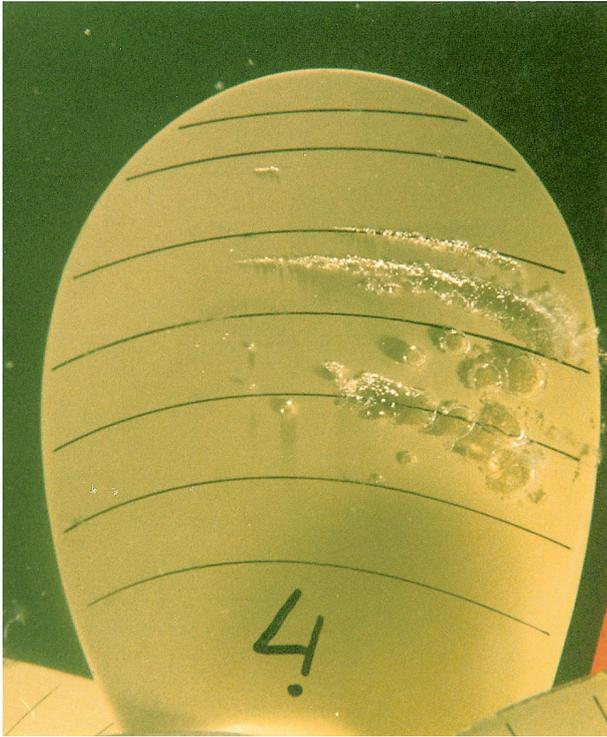
Figure 7.11: Bubble cavitation due to a turbulent spot with electrolysis
