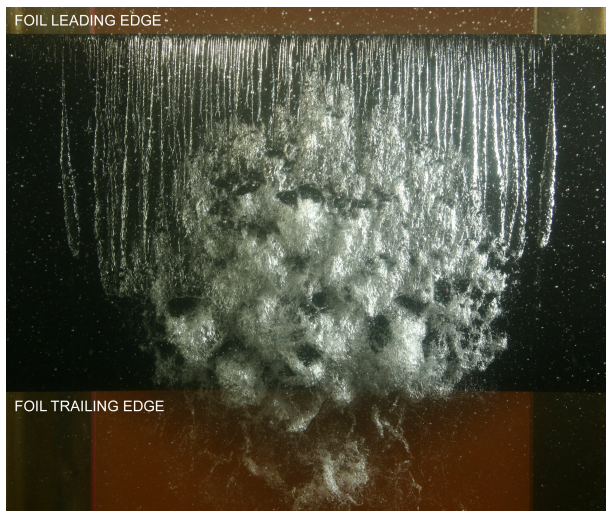
Figure 6.16: Regular but complex three dimensional shedding of a sheet cavity on a foil in steady inflow
