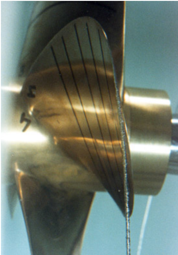
Figure 9.17: The cavitating core of a tip vortex behind a propeller
