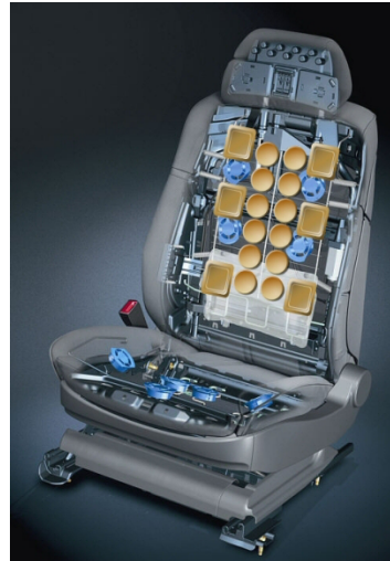
Figure 6. EMG recordings were made of the m. trapezius (upper four dots) and m. rhomboideus (lower four dots) to test the effect of the light weight massage system (right).
