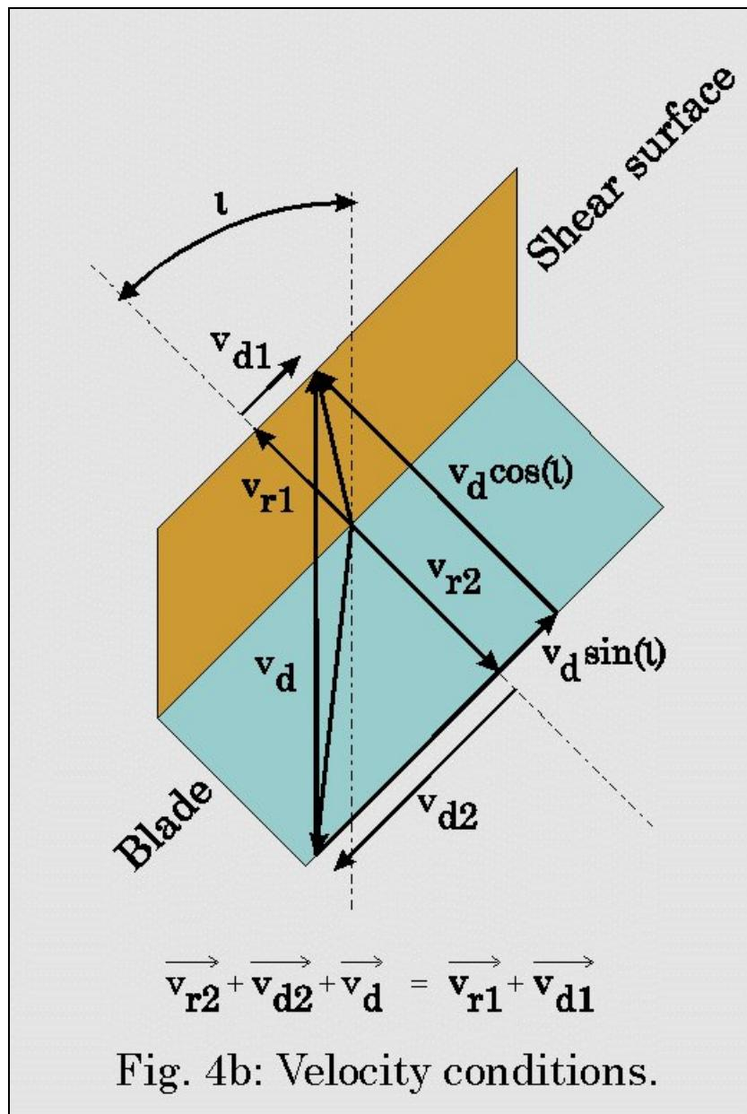
Fig. 4b: Velocity conditions.
