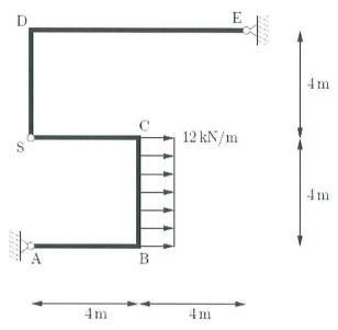
a) Graphically determine the direction of the reaction force in A.
