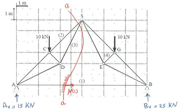
a) Determine the horizontal and vertical component of the reaction forces in A and B.
