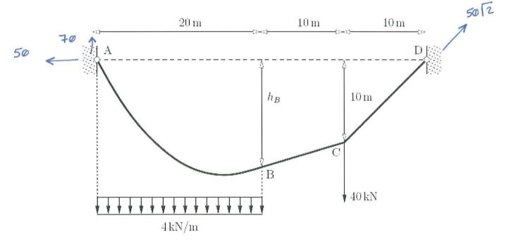
a) Determine the reaction forces in points A and D. Draw them in the figure as they act on the cable in reality.
