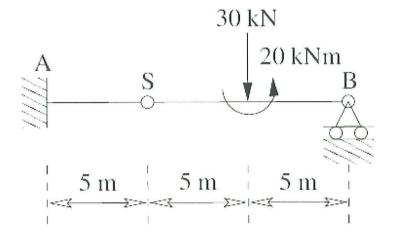
a) Using the principle of virtual work, calculate the reaction force in support B. Clearly indicate the virtual displacement field and the direction of the reaction force.
