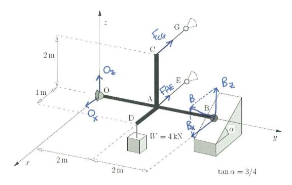
a) Calculate the reaction(s) in B. Draw them in the figure as they act on the structure in reality.
