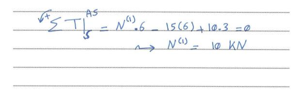
c) Determine by means of the method of sections the force in bar (2). Clearly indicate the section used.
