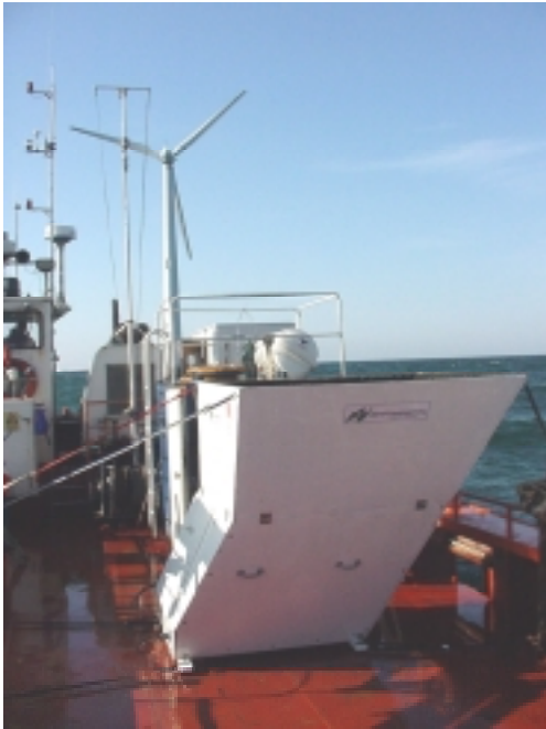
Figure 1. SODAR mounted on the ship 'Seaworker' at the Vindeby wind farm.
