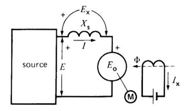
What is the horsepower at the output during this operation, neglecting the losses (iron, copper, etc)?
