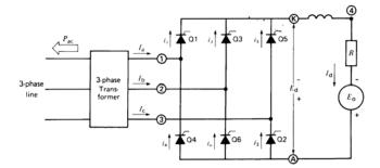
What is the active power delivered to the ac line (neglecting the transformer losses)?
