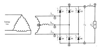
What firing angle is needed to generate 60V in inverter mode?
