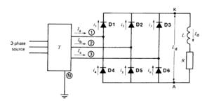
What is the power dissipated by all six diodes if the average voltage drop of each diode during the conduction period is 0.6V?
