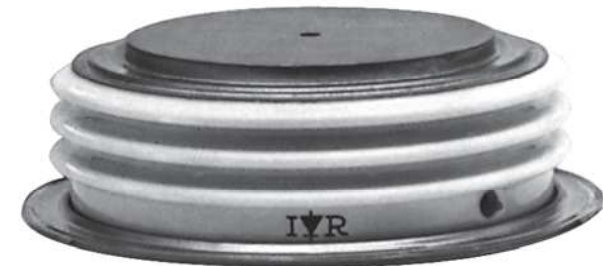
Figure 21.10 (continued) a. Average current: 4 A; PIV: 400 V; body length: 10 mm; diameter: 5.6 mm. b. Average current: 15 A; PIV: 500 V; stud type; length less thread: 25 mm; diameter: 17 mm. c. Average current: 500 A; PIV: 2000 V; length less thread: 244 mm; diameter: 40 mm. d. Average current: 2600 A; PIV: 2500 V; Hockey Puk; distance between pole-faces: 35 mm; diameter: 98 mm. (Photos courtesy of International Rectifier)
