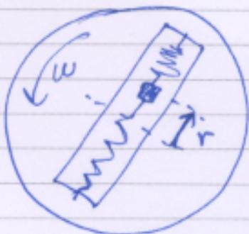
Displacement of mass w.r.t. centre is chosen as generalised coordinate
