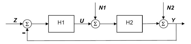
Closed loop configuration of two linear systems H1 and H2. Z external input; U: measured output of H1, Y: measured output of H2, N1: measurement noise, N2: output noise of H2.
