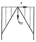
BSL Eq. 2.3-13, for flow of any fluid in a tube:
