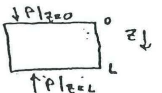
$z$  direction. Hence  $z=L$  term appears as negative term in momentum balance. Because this is steady-state, there is no accumulation term in balance. Momentum balance is
