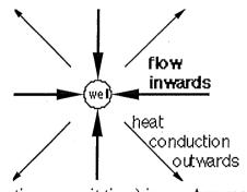
tion (in volume per unit thickness of formation per unit time) is  $q_0$ . Assume that the thermal conductivity k of the oil-saturated rock is known. At the surface of the well,  $T = T_w$ ; far from the well, the reservoir temperature is  $T_0$  ( $T_0 < T_w$ ). Assume both  $T_w$  and  $T_0$  are known.
