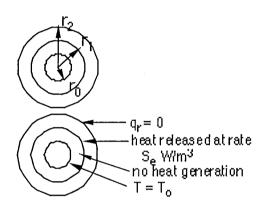
Se (in units W/m³). The inner layer  $(r_0 \le r \le r_1)$  has no heat generation, and the innermost surface can be assumed to be maintained by fluid at temperature  $T_0$ . The inner layer has thermal conductivity  $k^{01}$  and the outer layer has thermal conductivity  $k^{12}$ . Around the heating tape the experimentalist has placed insulation, so that there is no heat flux at the outer surface of this layer.
