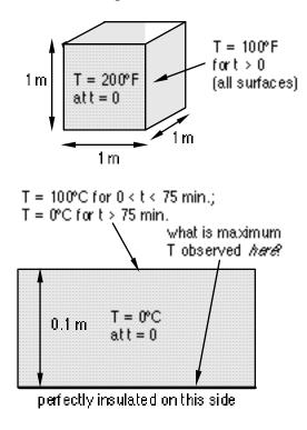
$$\rho = 3010 \text{ kg/m}^3 \qquad \begin{array}{c} \frac{\text{Properties of the slab}}{\text{C},^{\circ}_{p}} = 880 \text{ J/(kg K)} \qquad \text{k} = 1.21 \text{ W/(m °K)} \end{array}$$
