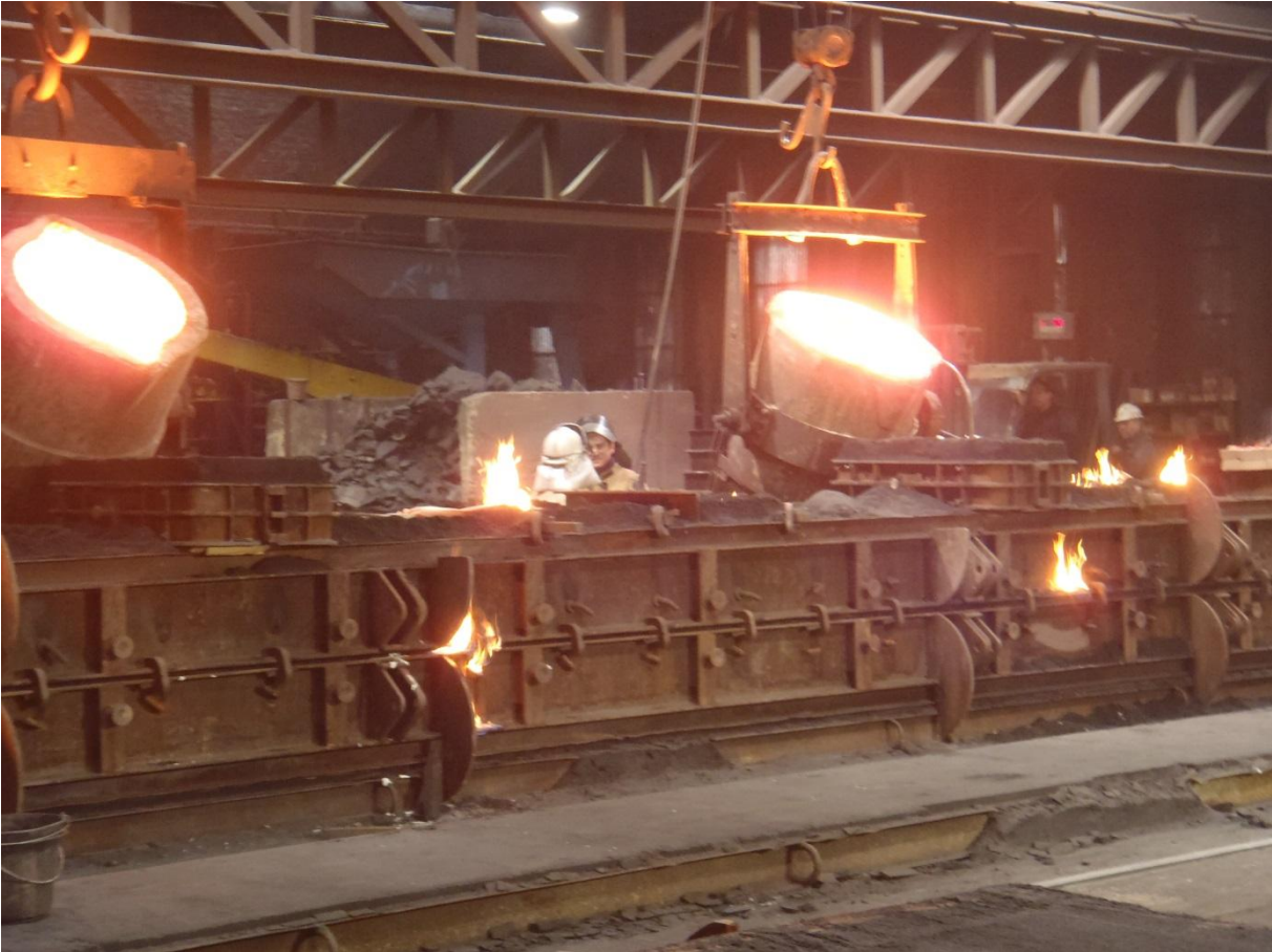
The pouring of iron in a mould.
