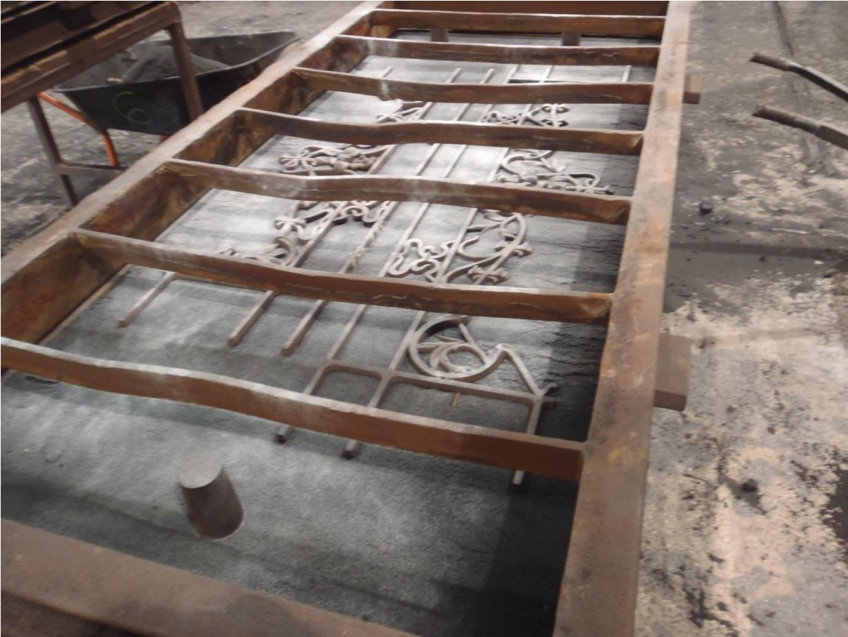
The Iron moulds with sand-shapes in it.
