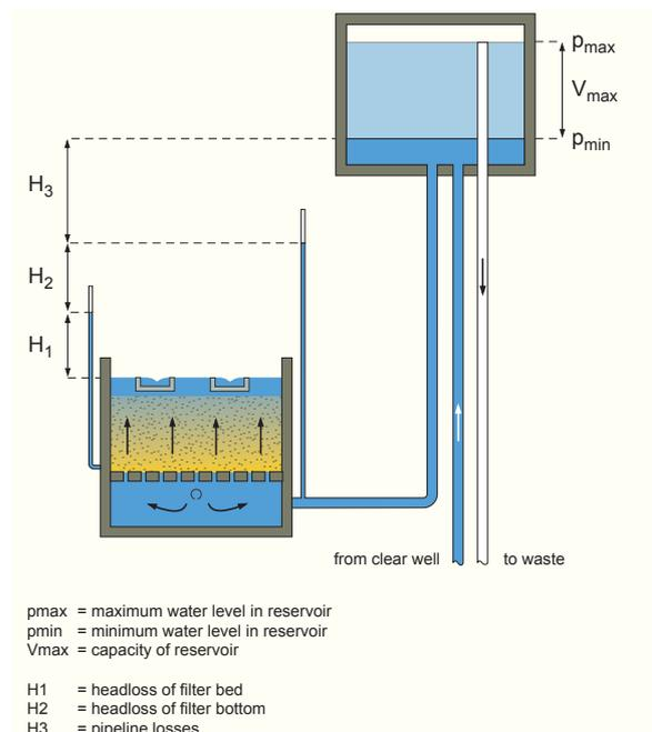
Figure 13 - Elevated water reservoir as backwash system
