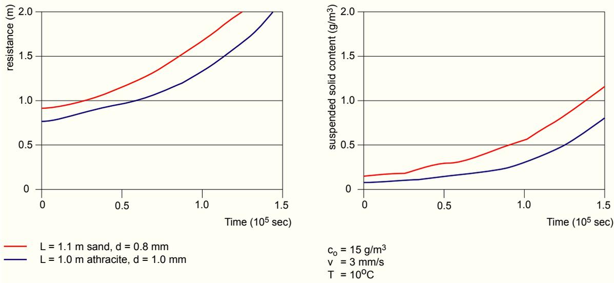
Figure 22 - Difference between single and multiple layer filtration for equal bed heights
