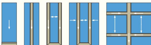
Figure 15 - A central backwash water trough
