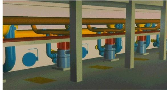
Figure 12 - Discharge pipes for backwash water are the largest pipes in a filter installation
