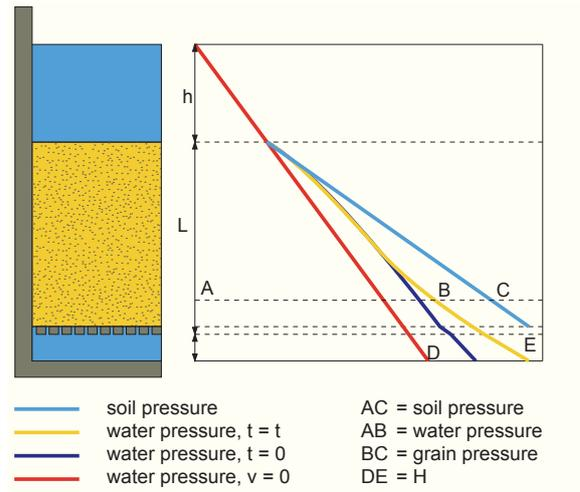
Figure 29 - Pressure distribution in an upflow filter
