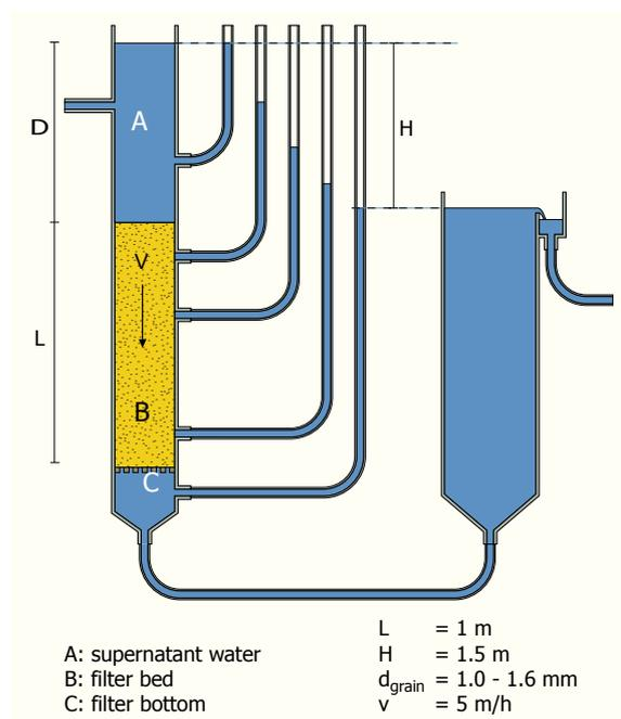
Figure 4 - Filtration, experimental setup
