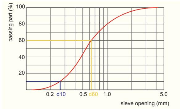
Figure 19 - Sieve curve of filter sand
