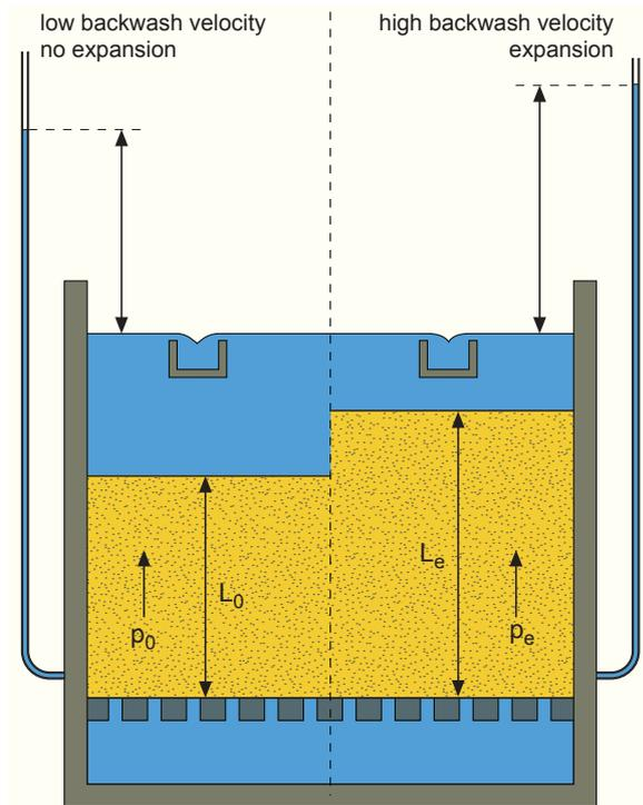
Figure 9 - A non-expanded and expanded filter bed
