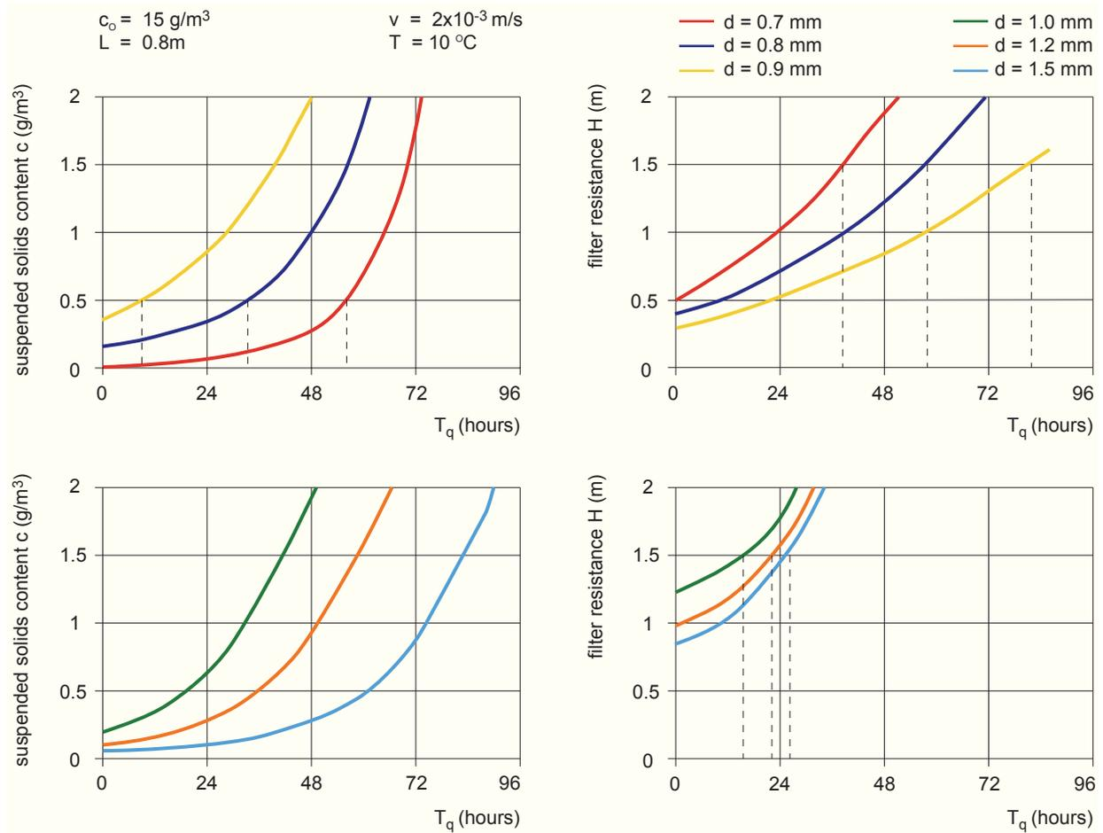
Figure 5 - Results of different filter runs to obtain an optimally functioning filter
