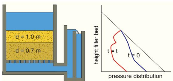
Figure 23 - Resistance build-up for a multiple layer filter
