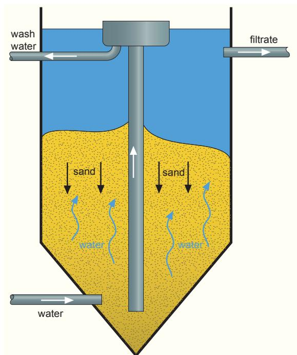
Figure 30 - Schematic representation of a continuous filter
