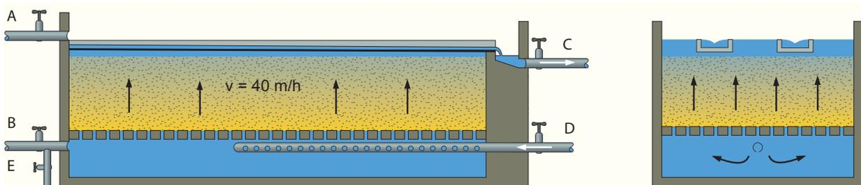
Figure 11 - Schematic representation of the backwash process
