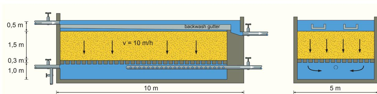
Figure 1 - Principle of rapid sand filtration (side and front view respectively)
