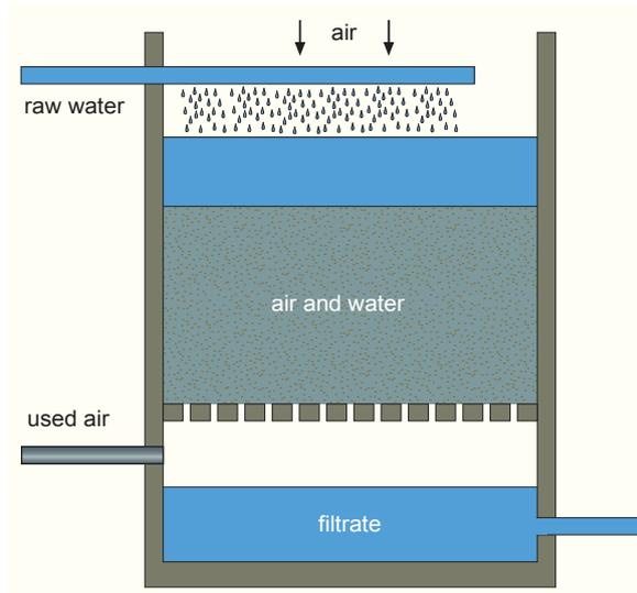
Figure 31 - Schematic representation of a co-current filter
