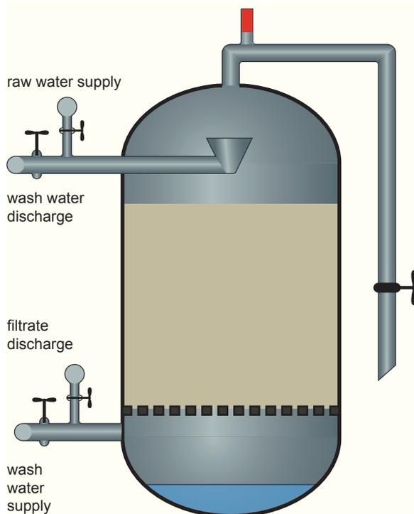
Figure 24 - Principle of pressure filtration
