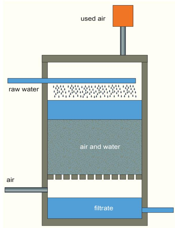
Figure 32 - Schematic representation of a counter-current dry filter
