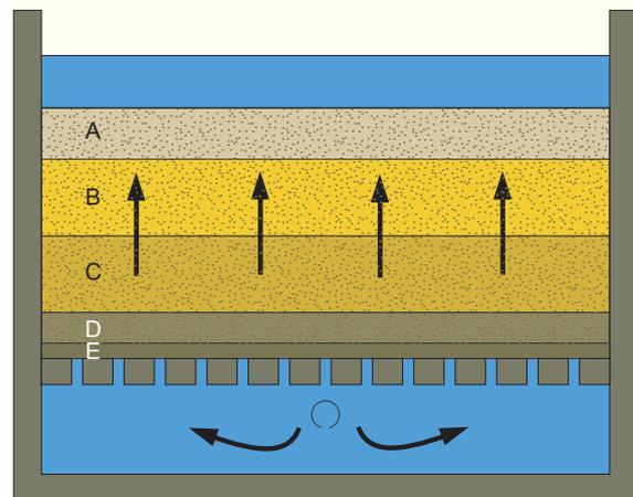
Figure 21 - Multiple layer filtration (upflow filter)
