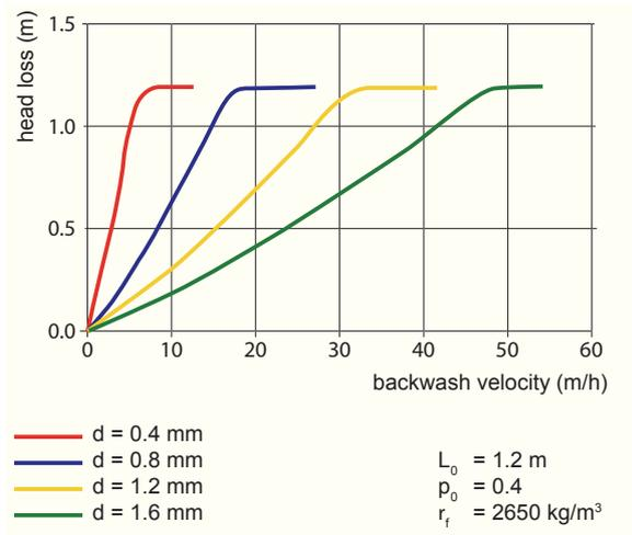
Figure 10 - Resistance during backwashing a sand filter bed with a height of 1.2 m as a function of the backwash velocity and grain diameter
