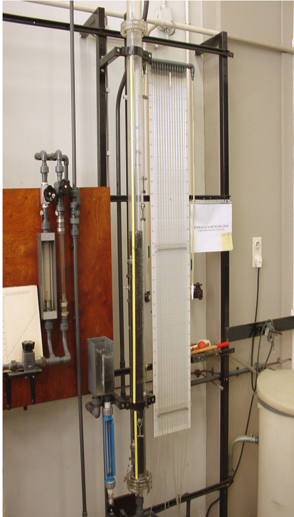
Figure 2 - Hydraulics of filtration in the laboratory
