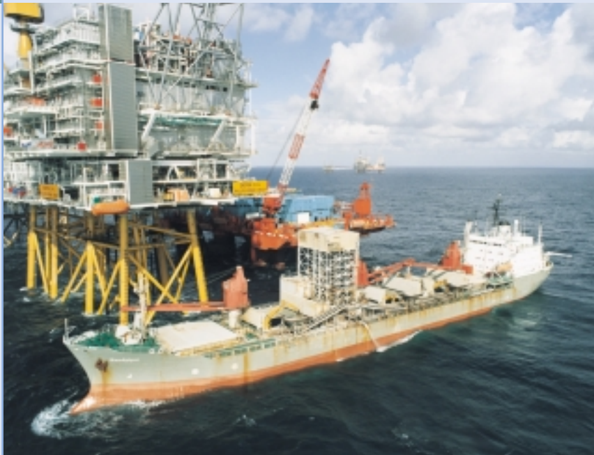
Grab on fallpipe vessel Seahorse that can be used to dredge down to 1,000 meters.
