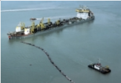
Land reclamation in Malaysia with the mega trailing suction hopper dredger W.D. Fairway.
