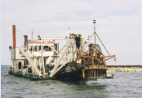
The specially developed environmental disc cutter Vecht, used for cleaning up the Ketelmeer.
